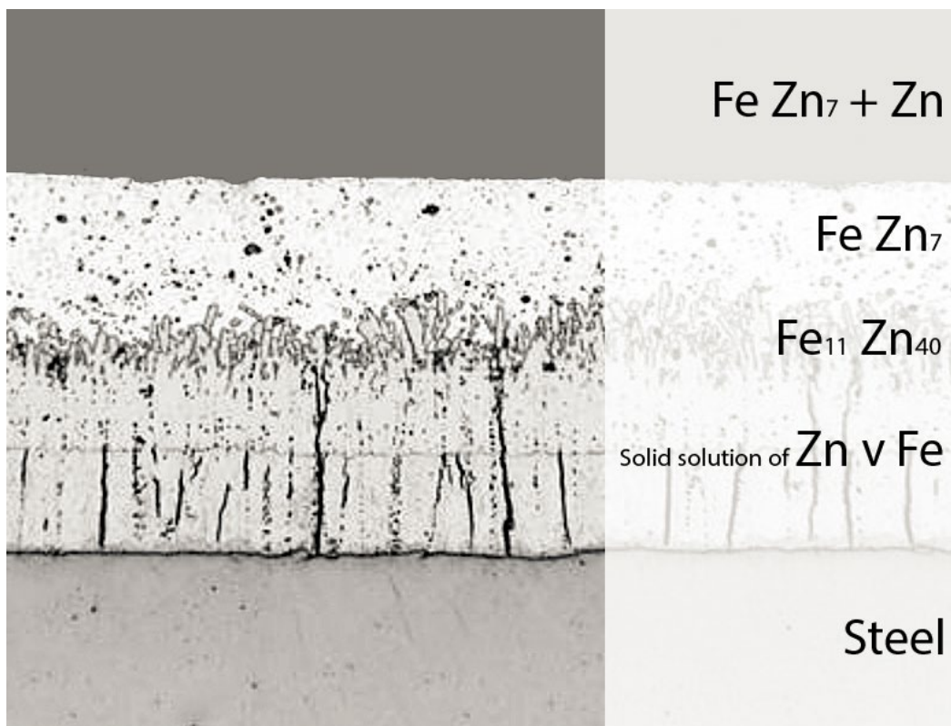
Coating cross-section, 200x magnification using an optical microscope
