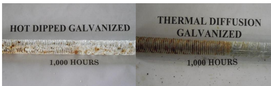
Figure 5 - Images from 1 000 hour neutral salt spray testing, conducted on the same grade of high tensile roof bolt material (Jeffrey, 2010)
