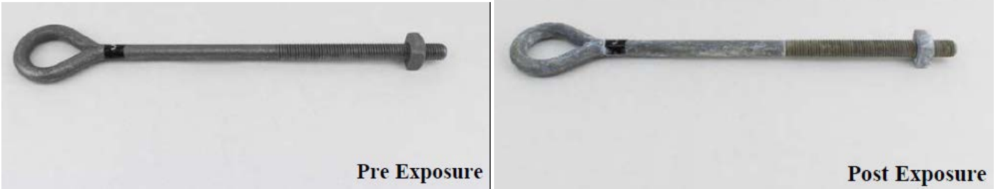
Figure 13: Corrosion results after 1000 hrs after full nut run ten times.
