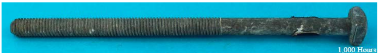
Figure 2: TZD after 1000 Hours Salt Spray
