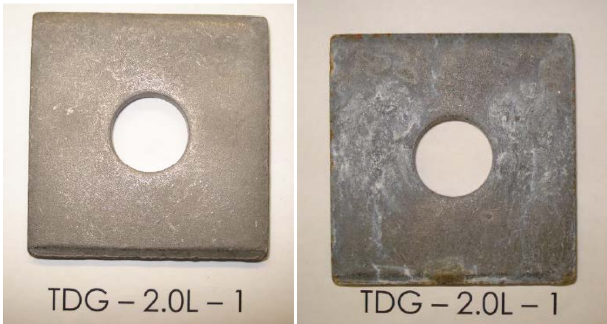
Figure 7: TZD sample 1 after 2.0L sand (left) and 500 hours salt spray (right).
