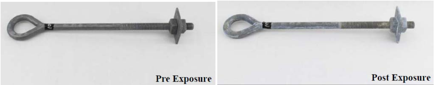
Figure 14: Corrosion results of J9412-T with washer clamped.
