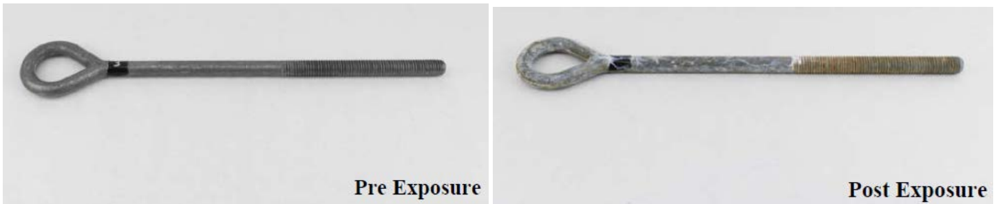
Figure 11: Corrosion results after 1000 hrs with residue wire brushed off.
