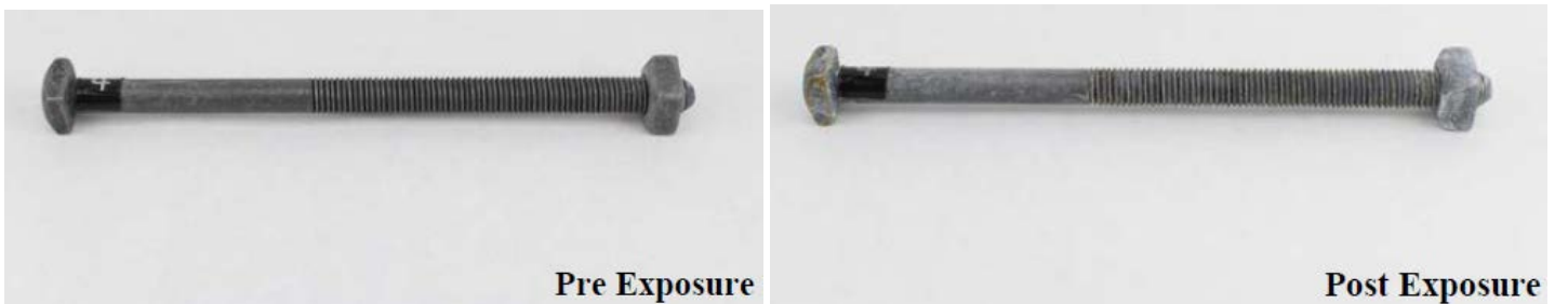
Figure 12: Corrosion results after 1000 hrs after nut run full on and off threads.
