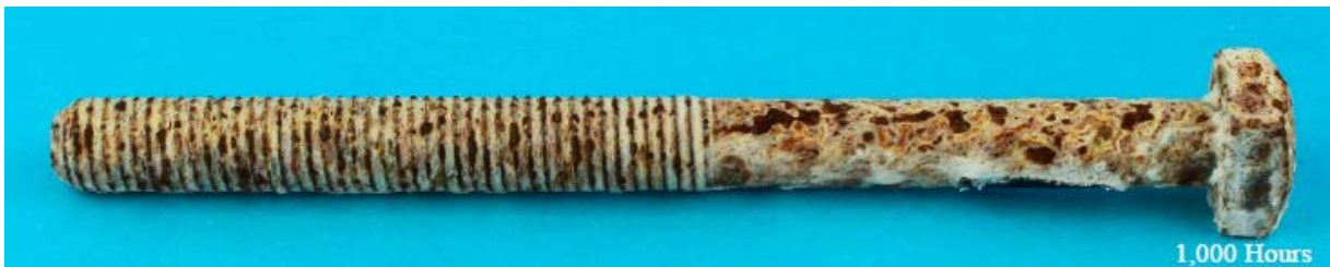
Figure 1: HDG after 1000 Hours Salt Spray
