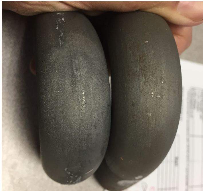
MacLean TZD bolts after bend test.
