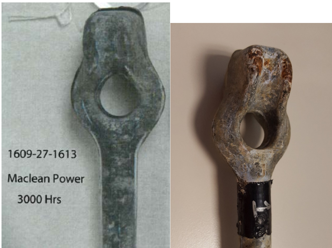
Figure 3: J8052-T after 3000 Hours Salt Spray and 4000 Hours Salt Spray (right)
