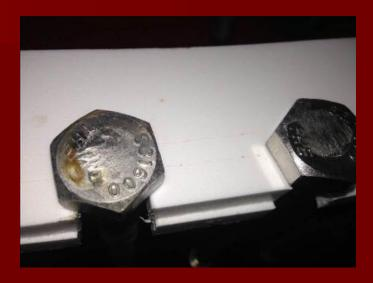
**<u>316 Status:</u>** Minor corrosion point on head and chamfer. No body corrosion Fully functional threads, no corrosion
