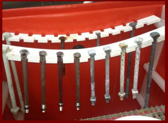
First row from left to right: ERX painted HDG, 316ss, 316ss, 304ss, 304ss, HDG silicate coated, HDG silicate coated, HDG, HDG, TDG
