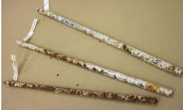
Figure 3 Traditional Hot Dipped galvanizing after 3000 hours in salt fog exposure
