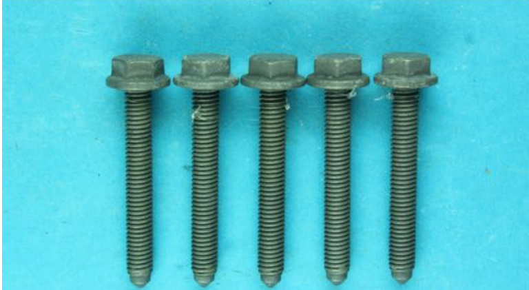
Grade 8 bolts for Automotive use (after 2040 hrs salt spray)
