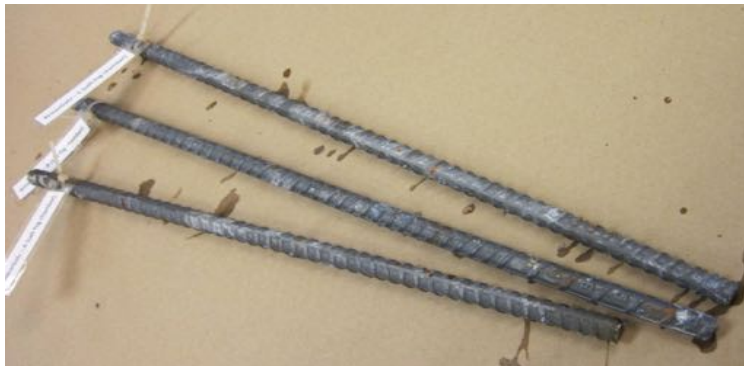
Figure 4 ArmorGalv® process after 3000 hours in salt fog exposure
