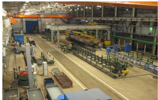
Large ArmorGalv® system, coating Structural elements up to 12m (40ft) long.
