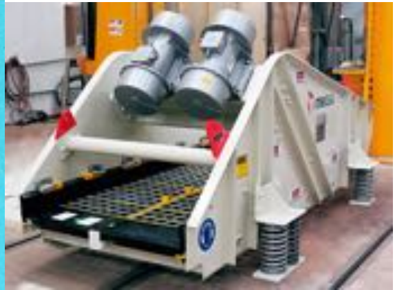
Springs on a vibratory mining screen coated with ArmorGalv® for corrosion protection and fatigue performance.
