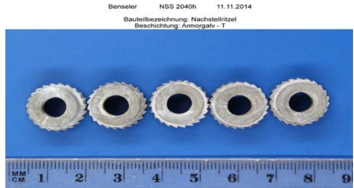
Sintered steel ratchet wheels (2040 Hrs salt spray)
