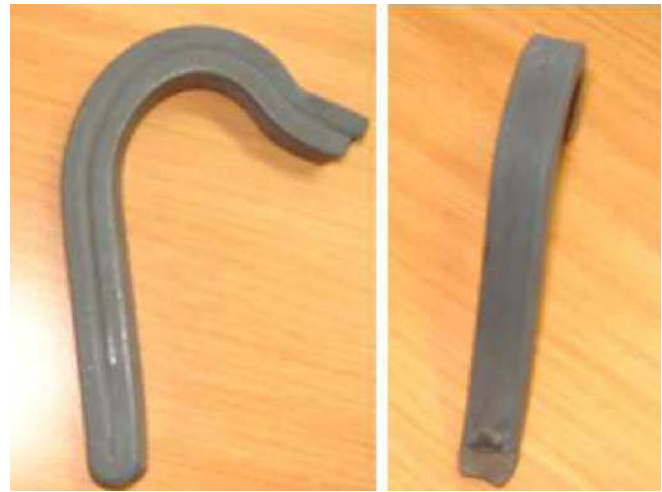
Fig. 1 Part: forged steel with tight crack
