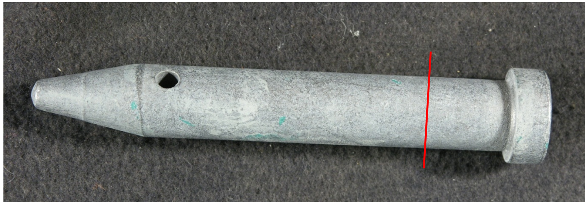
Figure 1 Bolt as received. Red line indicates cross section taken for examination.
